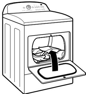
Open the door by pulling on the handle. Place laundry in the dryer. Add a dryer sheet to wet load, if desired. Close the door.
