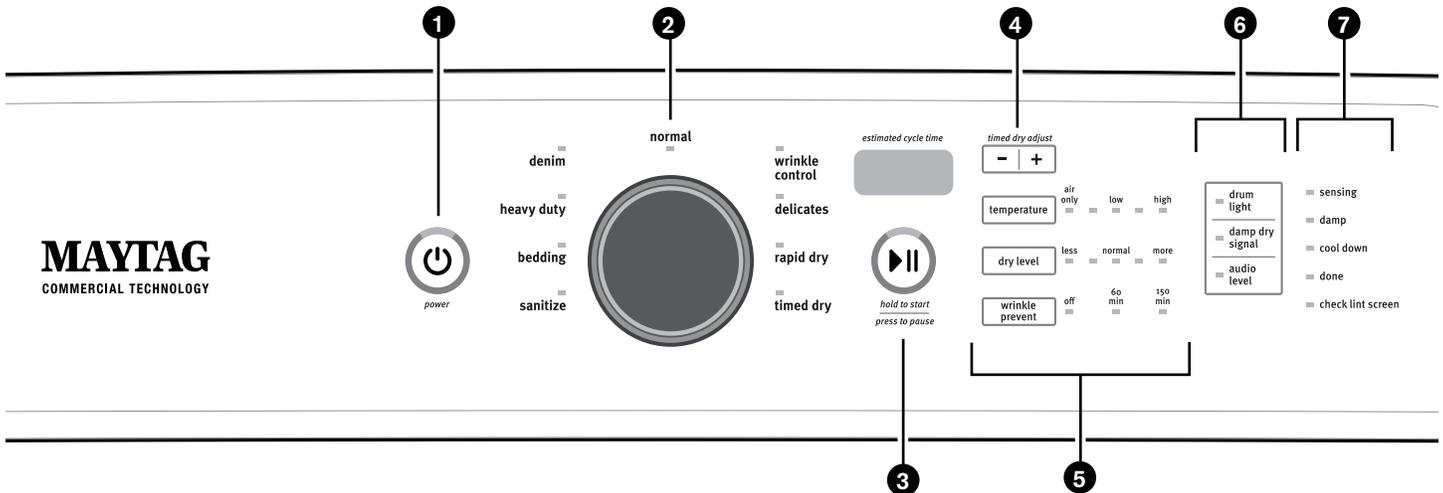
**NOTE:** The control panel features a sensitive surface that responds to a light touch of your finger. To ensure your selections are registered, touch the control panel with your finger tip, not your fingernail. When selecting a setting or option, simply touch its name.
