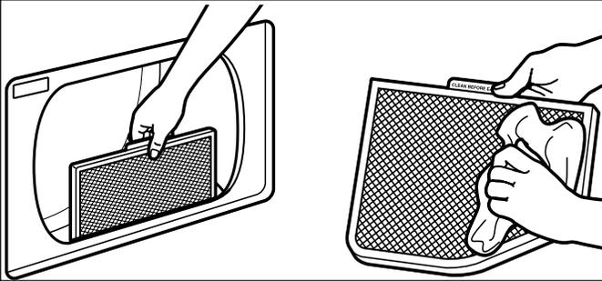
Clean the lint screen before each load. Pull the lint screen out of its holder. Roll lint off the screen with your fingers. Do not rinse or wash screen to remove lint. Push the lint screen firmly back into place.
