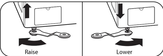
2. Loosen the locknuts on all four leveling feet with the wrench until you can adjust the feet (wrench appearance may vary). Use the wrench to turn the feet clockwise to raise the washer, and counterclockwise to lower the washer. Using a level, adjust the feet until the washer is level from side to side and front to back. Make sure that all four feet are in firm contact with the floor.
