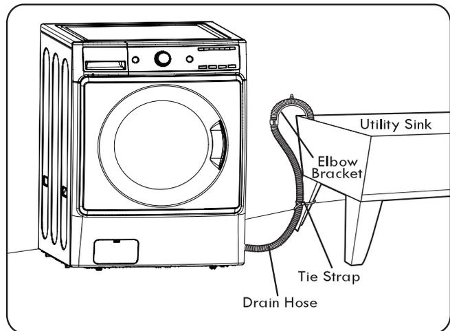
The elbow bracket should be installed near the end of the drain hose. Hang the end of the drain hose over the side of the utility sink. Use a tie strap to secure the drain hose in place.
