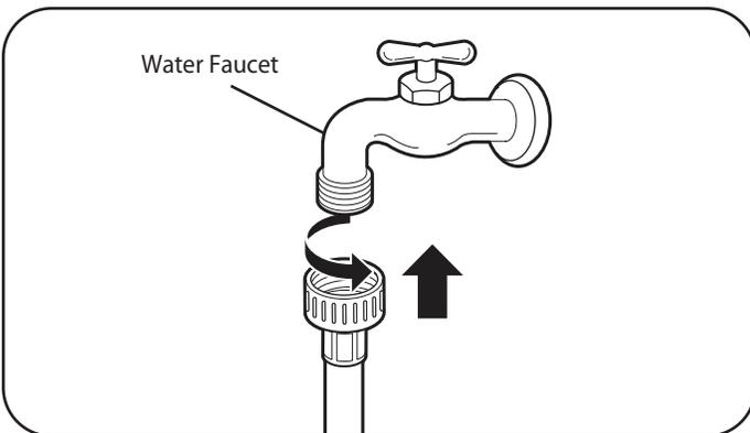
2. Connect the water supply hoses to the HOT and COLD water faucets tightly by hand and then tighten another 2/3 turn with pliers.
