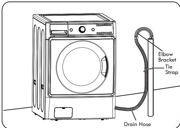
Install the end of the drain hose into the elbow bracket. Do not extend the drain hose more than 4 inches past the end of the elbow bracket. Use a tie strap to secure the drain hose in place.
