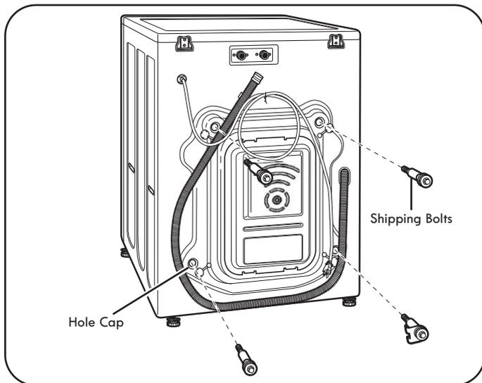
2. Remove the bolt assemblies by wiggling them slightly while pulling.
