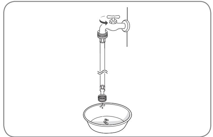
3. Always run a gallon or two of water through each inlet hose to flush dirt, scale and other debris out of the water lines. Doing so will help prevent future problems with clogged filter screens, and will also allow you to verify which water line is hot and which is cold.
