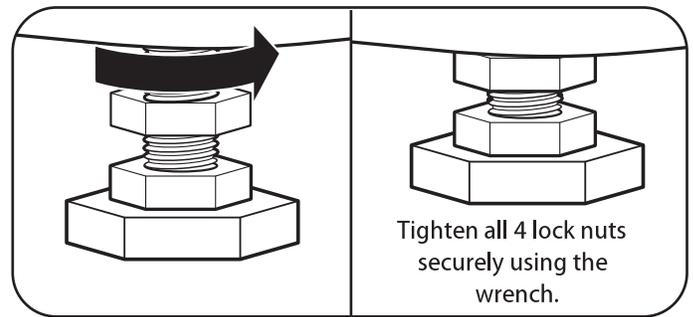
3. Once the washer is level from side to side and front to back, use the adjusting wrench to tighten all four lock nuts securely to prevent the legs from getting out of adjustment during operation. Make sure that all four leveling feet are in firm contact with the floor.
