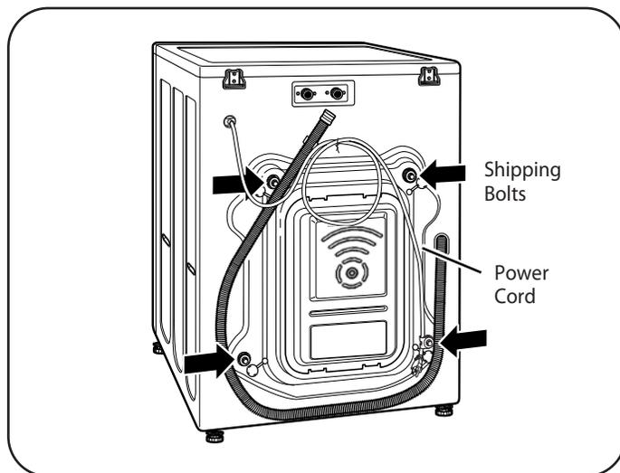
1. Starting with the bottom two shipping bolts, use the wrench (included) to fully loosen all four shipping bolts by turning them counterclockwise.
